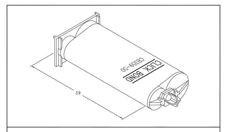
CB359 EPOXY ADHESIVE IN DUAL PACK CARTRIDGE
